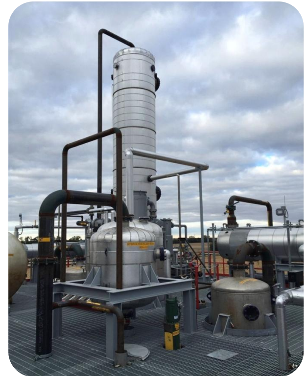
The process finishes the biodiesel by distillation, thereby providing a clear as water biodiesel that will not change the typical ULSD diesel fuel color.
